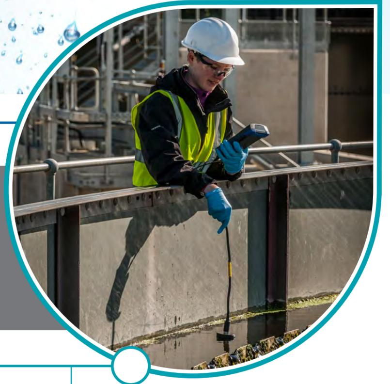
BOD-Wader systems provide real-time, highly sensitive, *in situ* assessment of Biological Oxygen Demand within water systems, informing on the impact of biodegradable substances.
