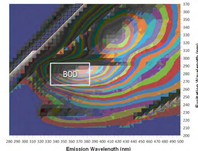
Fluorescence map of an environmental water sample spiked with Tryptophan, indicating BOD-Station measurement window
