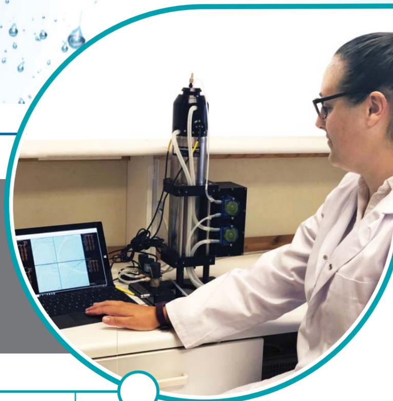
Act2 & the FastOcean FRR fluorometer can be combined to produce a highly automated system for probing oxygenic photosynthesis by phytoplankton
